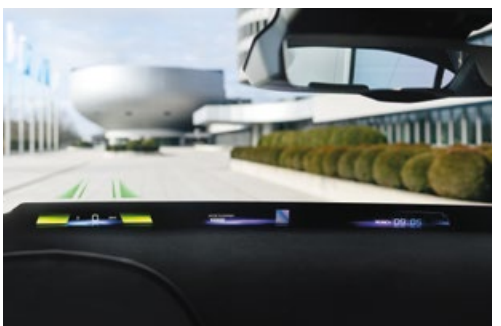
»Panoramic Vision«: the new head-up display from BMW
