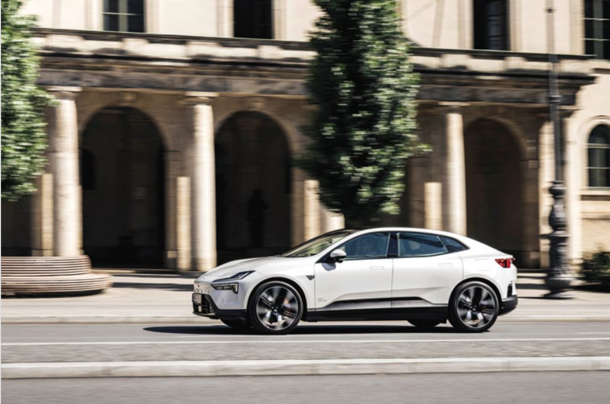
The Polestar 4, an SUV coupe, has no rear window; instead, there is a rear camera.
