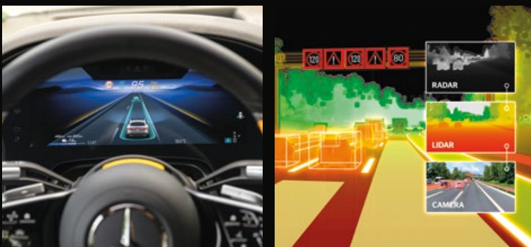
Left: Drive Pilot from Mercedes enables autonomous driving at level 3 up to a speed of 95 km/h from this spring.
