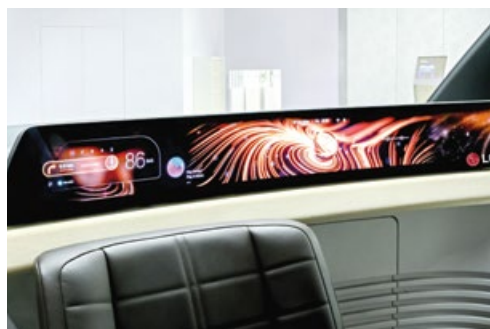
The largest automotive display to date comes from LG and has a screen diagonal of 1.45 metres.
