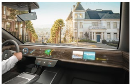
Continental ShyTech Display: operating options only become recognisable when a hand approaches.
